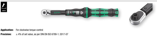
Design: With ¼" hex drive, reversible ratchet, 45 teeth; easy setting and saving of the desired torque value, with audible and tactile locking when the scale values are reached (fine scale only in Newton meters), audible and tactile release mechanism when the set torque value is reached
