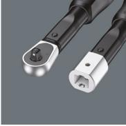
The Click-Torque wrenches are available for clockwise torque-controlled tightening with a reversible ratchet  $(\frac{1}{4}^{"}, \frac{3}{8}^{"}, \frac{1}{2}^{"}$ and  $\frac{3}{4}^{"}$  drive) or for insert tools (9x12 mm, 14x18 mm) for torque ranges from 2.5 Nm to 1000 Nm.
