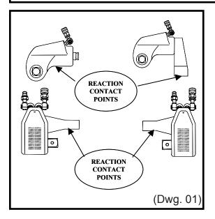
Make sure the reaction arm is positioned correctly. (Refer to Dwg. 01).
