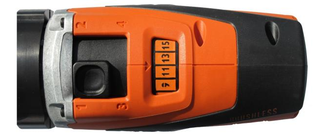
Set the desired torque using the calibration certificate: first determine the gear and setting with the aid of the tables on the last page of the calibration certificate. Then select the gear by means of the black sliding switch. Gear 1 is the slowest speed and Gear 4 the fastest. The sliding switch must not be positioned in the centre but has to fully click into place; otherwise the device will jam. Only change the gear when the device is not moving.
