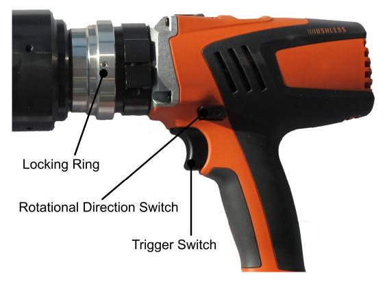
The diamond-shaped reversing switch is indicated on either side with an arrow for the specific direction of rotation. Pressing the reversing switch changes the direction of rotation, see Figure. Make sure that the reversing switch has clicked firmly into place to the extreme left or right. Only change the direction of rotation when the device is not moving.
